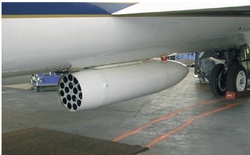
0344-F0009 Figure 9 Remote-controlled GPS dropsonde launcher system installed on the NASA ER-2 high-altitude weather research aircraft.
